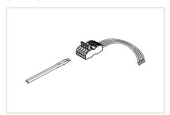
Connect the wires coming from the amplifier to the SnapConnect™ on the rear speaker part.
