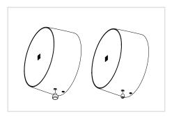
The NELO706V includes two knobs for volume adjustment. The protruding knob is assembled by default and allows easy adjustment by hand. This is recommended for frequent volume changes. A second flush knob with screwdriver notch is included and recommended for permanent settings, or when rare and non user configurable adjustments are required.
