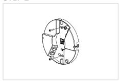
The wall part has to be assembled to the provided location on the wall or ceiling. This is done through knocking out the provided areas (teardrop holes) for the fasteners. Choose the fasteners depending on the mounting surface (concrete, wooden, steel, ...) The distance between both mounting positions is 130 mm.
